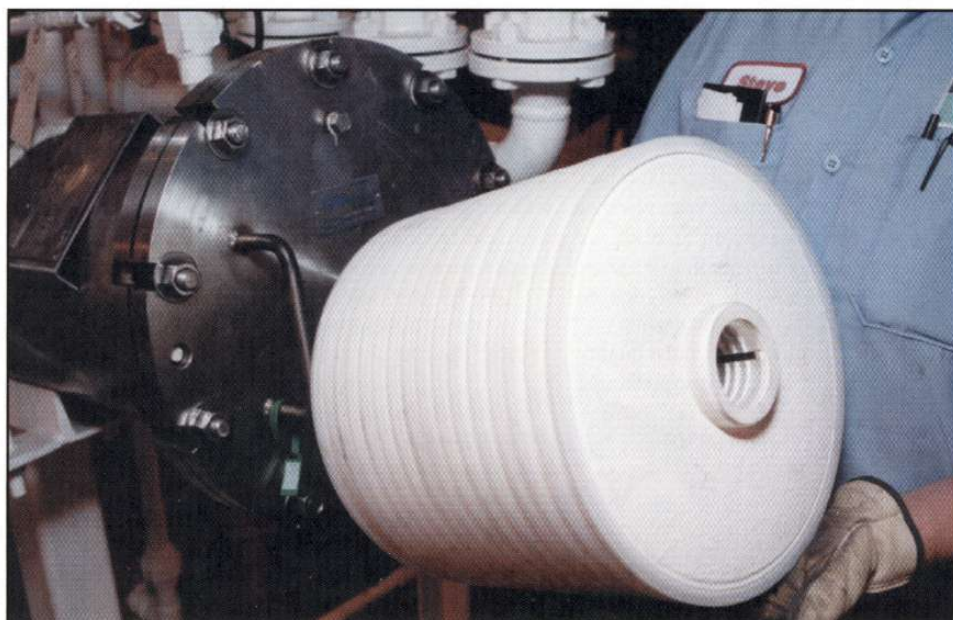
The disc pack cartridge element shown here is precoated with a filter aid to assist in the removal of small particles or second-phase liquids. This is a potential replacement technology for filter presses.
